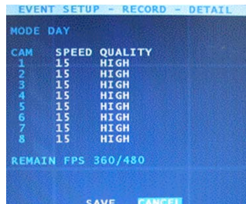
Figure 34 – Event Setup – Record - Detail
