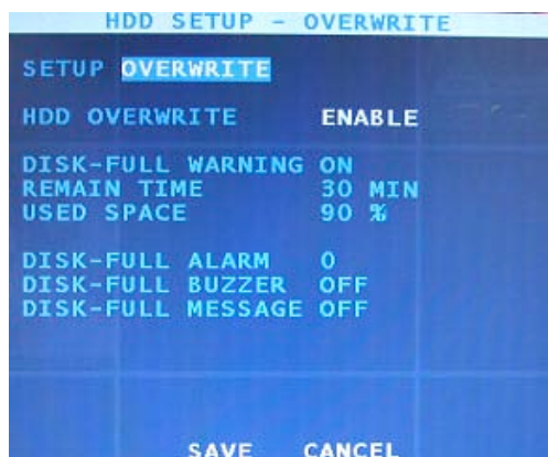
Figure 12 – HDD Setup – Overwrite.
