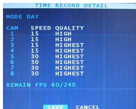
Figure 27 – Time Record Setup (Speed & Quality).
